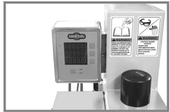
Figure 24. DRO magnetically mounted to mill headstock.
