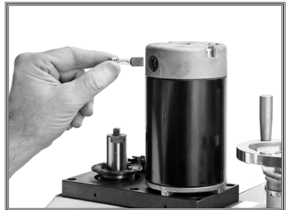
Figure 49. Inserting new motor brush.
