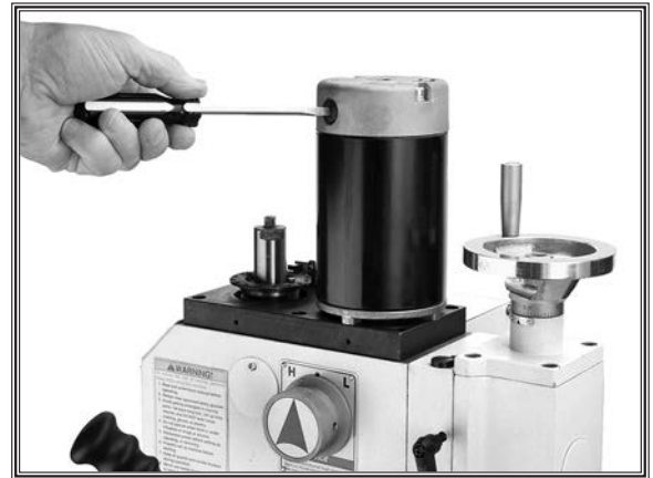
Figure 48. Removing motor brush cap.
