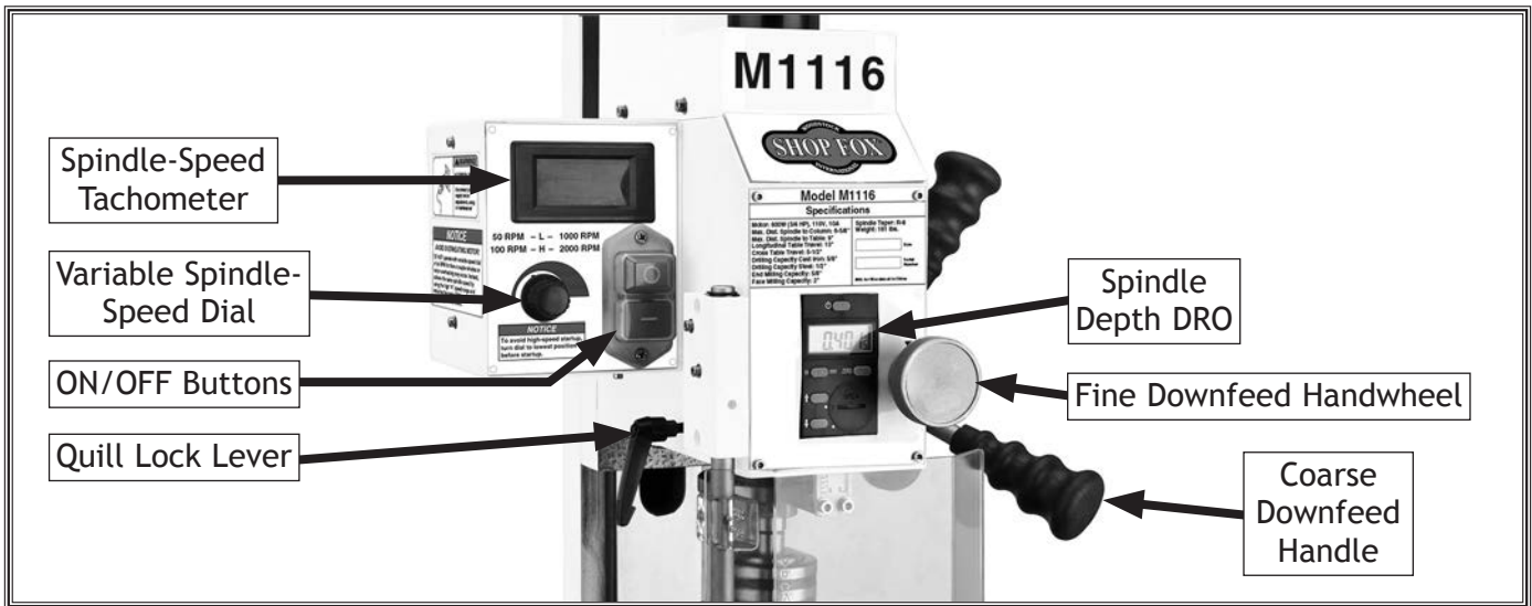
Figure 2. M1116 headstock identification.
