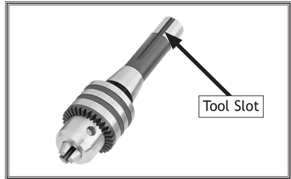
Figure 28. 1-13mm drill chuck joined with R8 arbor.
