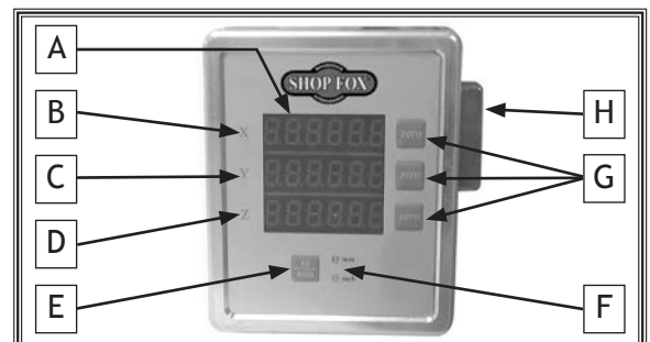
Figure 27. DRO controls and display.
