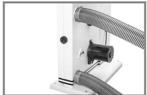
Figure 20. Dust port connected to dust collection system.
