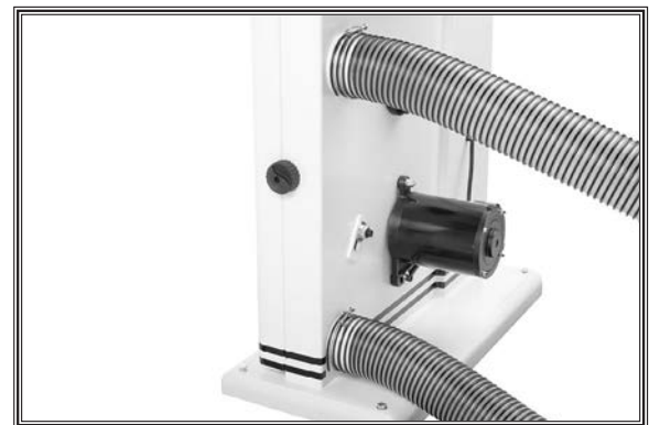
Figure 16. Dust hoses connected to dust ports.
