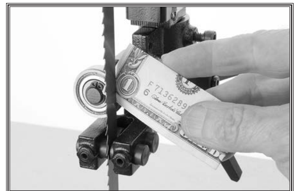
Figure 27. Dollar bill folded twice to make a quick 0.016" gauge.
