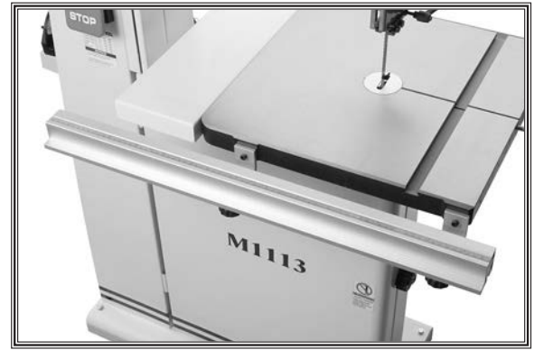
Figure 17. Scale installed on front fence rail.
