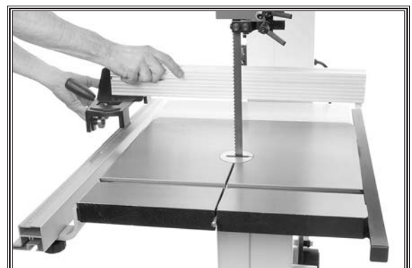
Figure 16. Installing fence onto rails.
