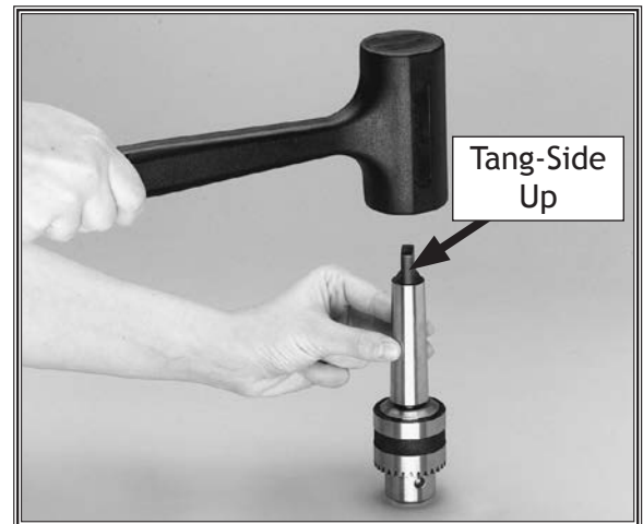
Figure 21. Seating the arbor into the chuck.
