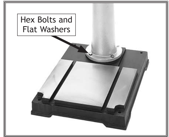
Figure 8. Column secured to base.
