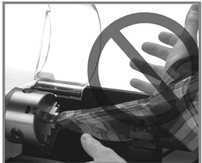
Figure 5. Never use the lathe with loose fitting clothing, or you may become entangled.
