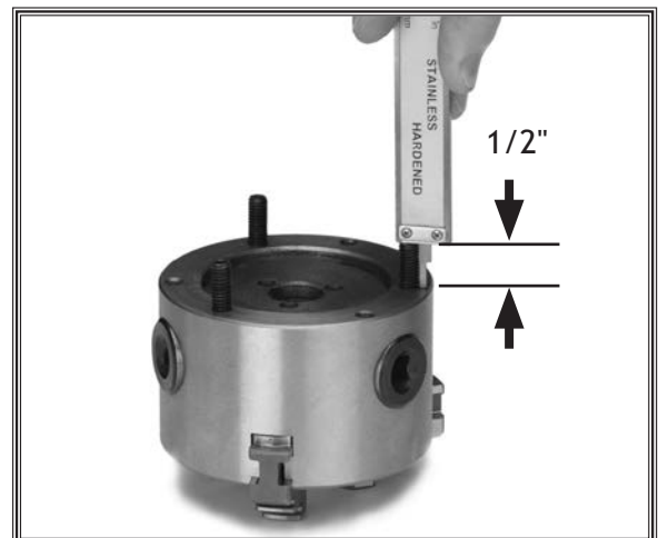
Figure 5. Checking stud protrusion.
