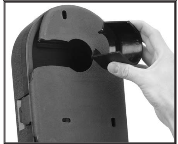
Figure 19. Installing the bearing guard.
