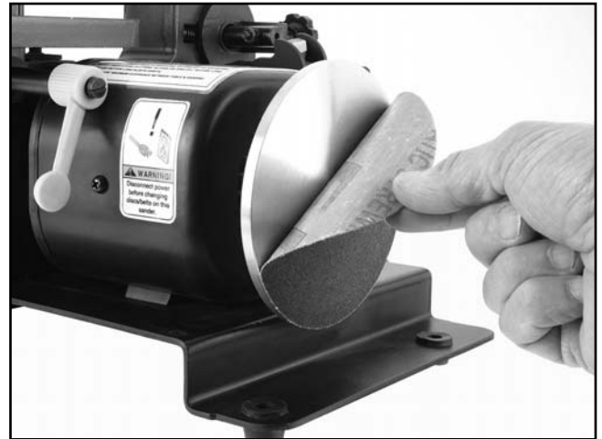
Figure 17. Sanding disc removal and Installation.
