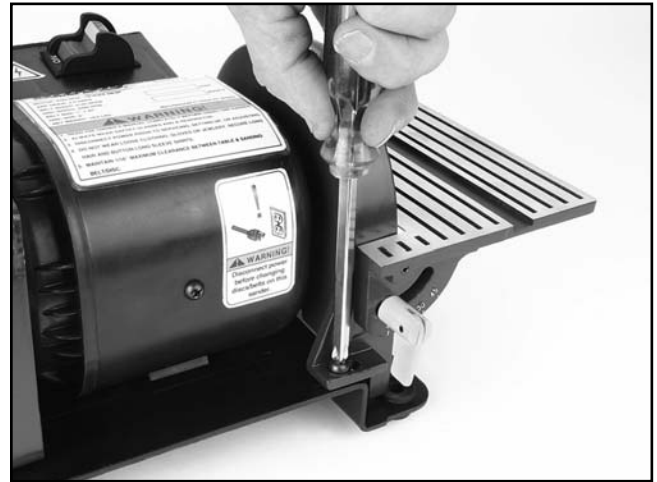
Figure 5. Disc guard and table installation.
