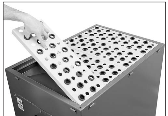
Figure 7. Installing downdraft plates.
