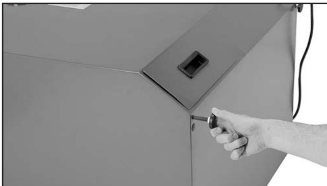
Figure 5. Installing foot pads.
