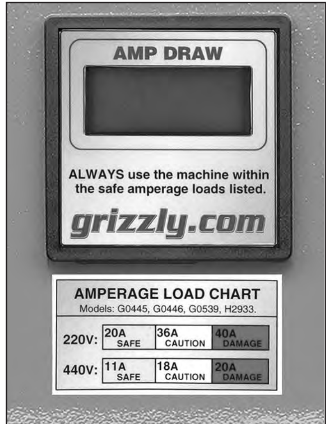
Figure 17. Typical amp draw meter and load chart.
