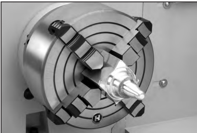
Figure 24. Generic picture of non-cylindrical workpiece correctly mounted on the 4-jaw chuck.
