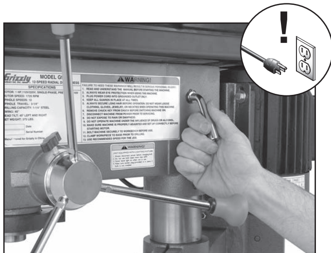
Figure 21. Using the belt tension lever.
