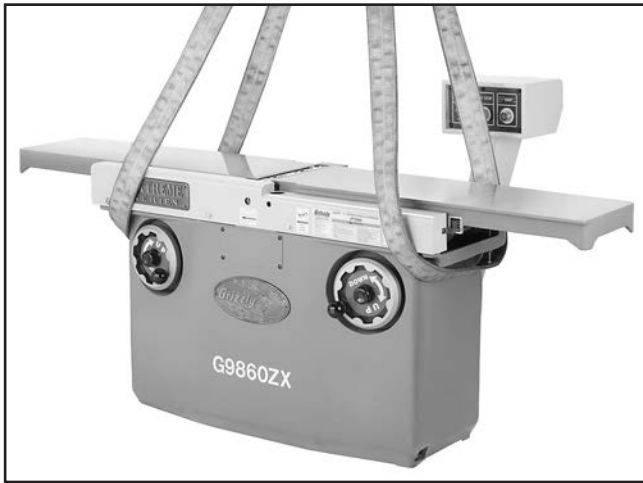
Figure 16. Lifting straps properly positioned.
