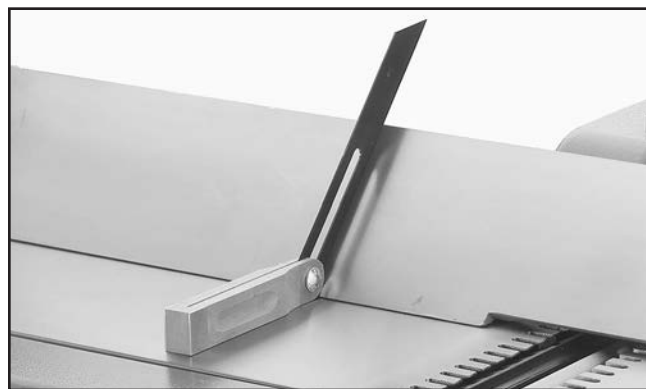
Figure 66. Setting the fence to 45° (135°), with the cutterhead guard removed for clarity.
