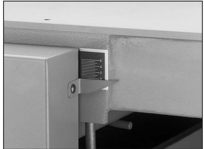
Figure 75. Depth of cut scale and pointer.
