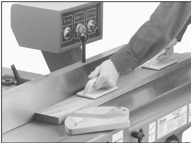
Figure 40. Example of surface planing with the jointer.
