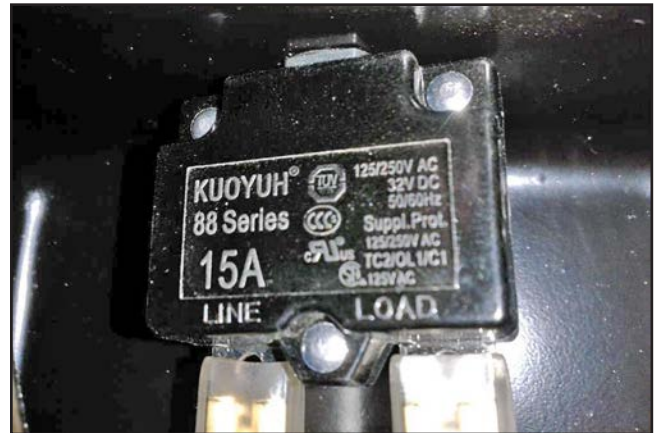
Figure 52. Circuit breaker wiring.
