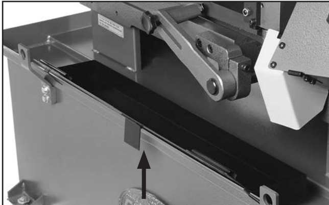
Figure 10. Chip tray installed.
