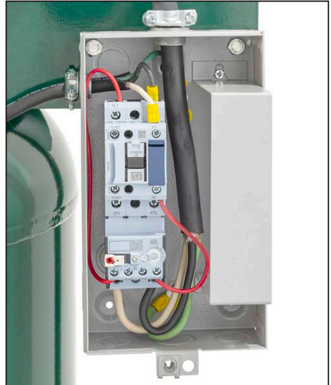
Figure 64. Magnetic switch box wiring.
