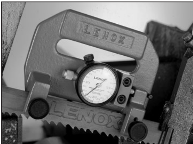
Figure 29. H5408 blade tensioning gauge.
