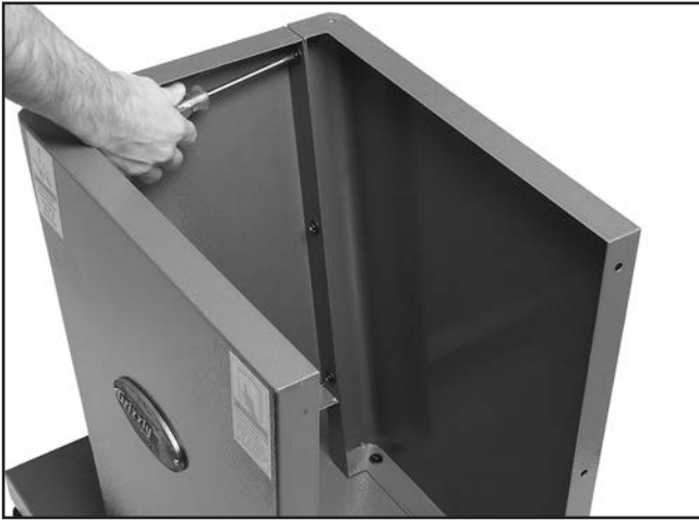
Figure 8. Left Panel installed.
