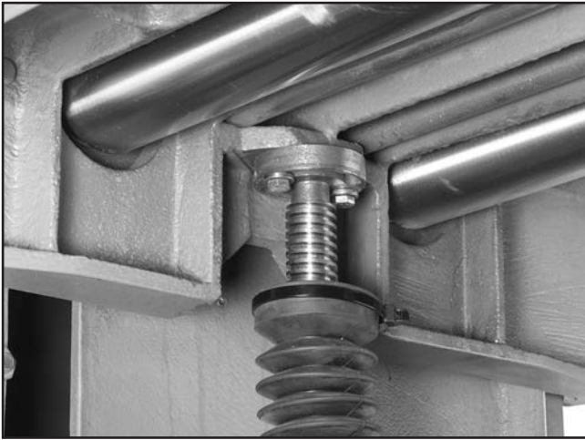
Figure 14. Column adjustment flange underneath table.
