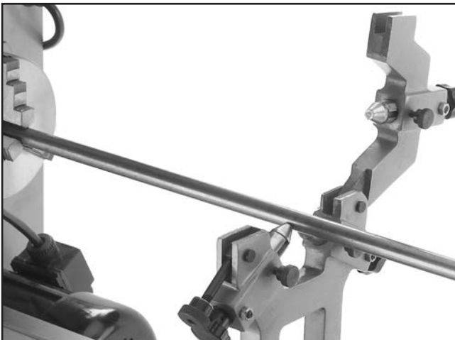
Figure 33. Loading the workpiece into the steady rest.
