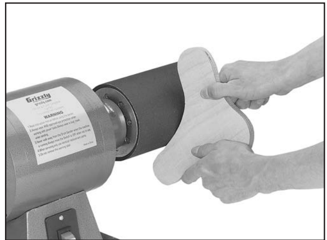
Figure 1. Typical drum sanding operation.
