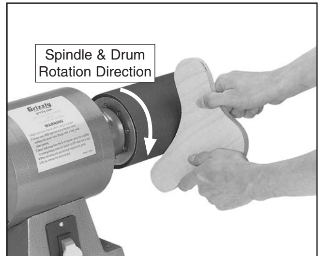
Figure 15. Typical drum sanding operation.
