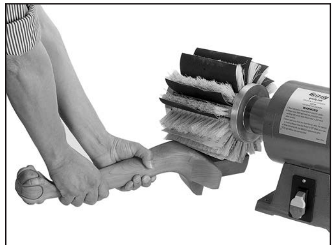
Figure 2. Typical flap sanding operation.
