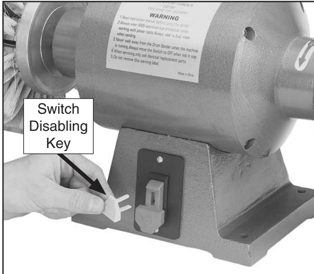
Figure 14. Removing the ON/OFF switch disabling key.
