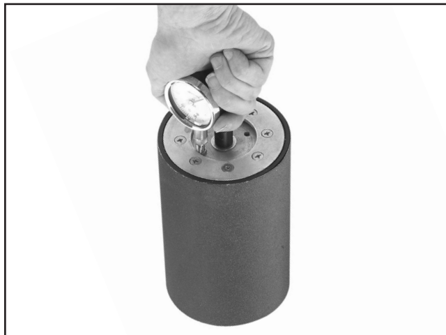
Figure 12. Checking sanding drum air pressure.
