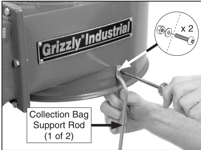
Figure 10. Attaching collection bag support rods to collector.
