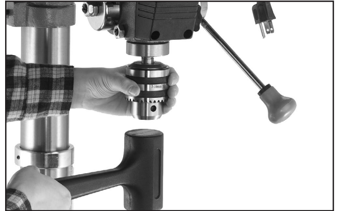
Figure 23. Seating chuck into spindle. (Note retracted jaws.)
