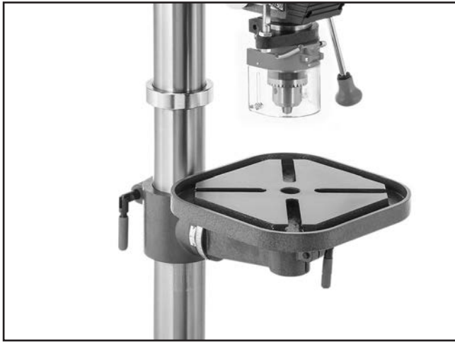
Figure 23. Table installed (G7943 shown).
