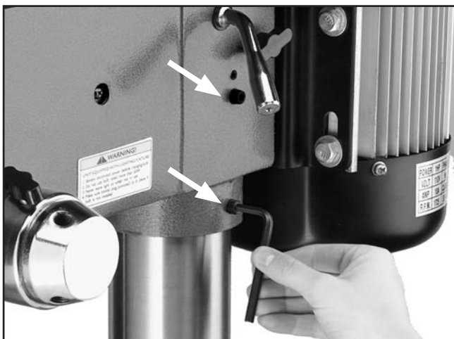
Figure 20. Securing headstock to column.
