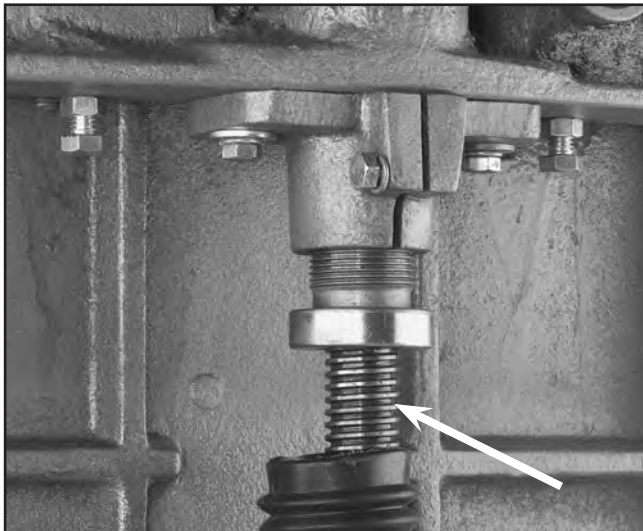
Figure 27. Pull down rubber boots under the table to expose the worm gears that raise and lower the table.
