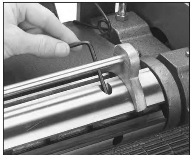
Figure 8. Adjusting knife height.
