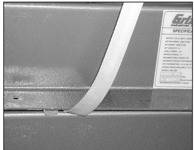
Figure 6. Chock in place so lift strap can be removed.
