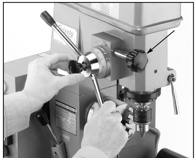
Figure 27. Move the handle while depressing knob.
