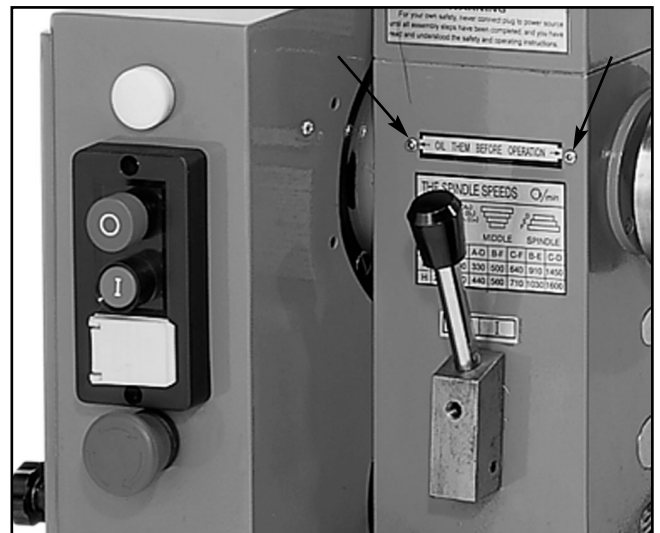
Figure 53. Gearbox lubrication points.
