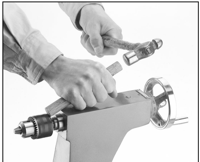
Figure 12. Seating the arbor and drill chuck.
