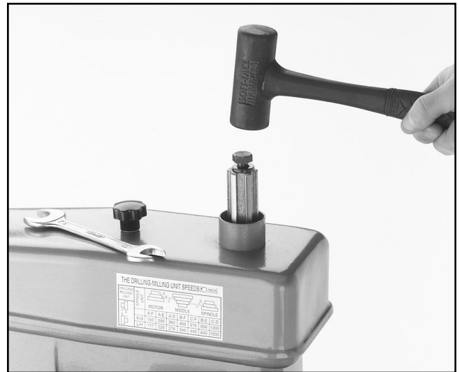
Figure 11. Removing drill chuck.
