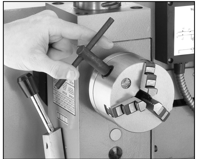
Figure 6. Rotate chuck key to open/close jaws.
