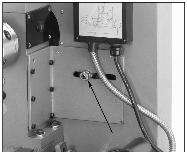
Figure 17. Loosen this nut to adjust pulley.
