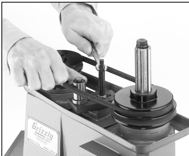
Figure 26. Loosen stud to pivot belt tensioner.
