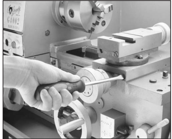
Figure 31. Adjusting the cross-slide gib.
