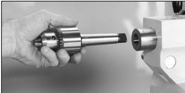
Figure 33. Example of drill chuck installation.
