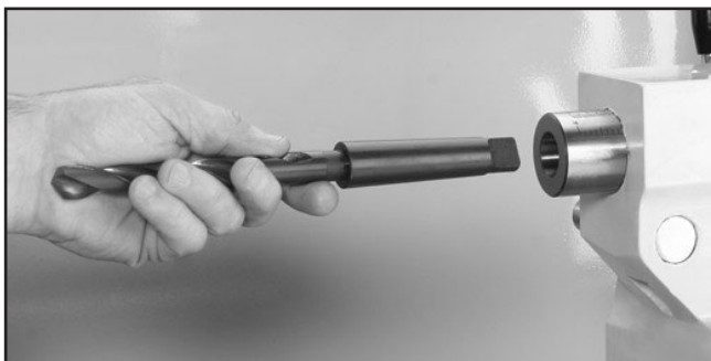
Figure 34. Example of drill bit installation.
