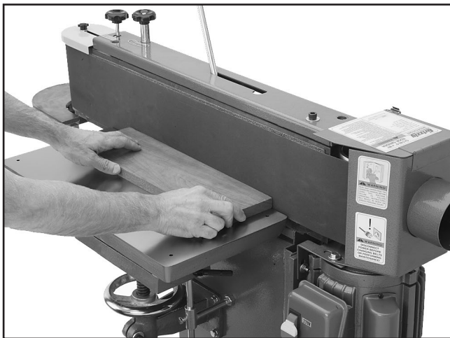
Figure 37. Typical edge sanding method.
