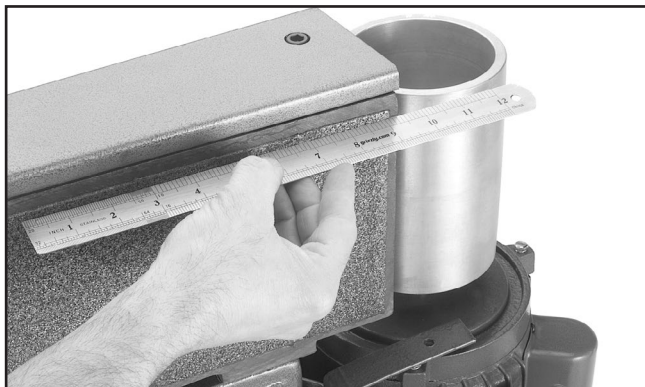
Figure 55. Example of checking top of platen-to-roller.
