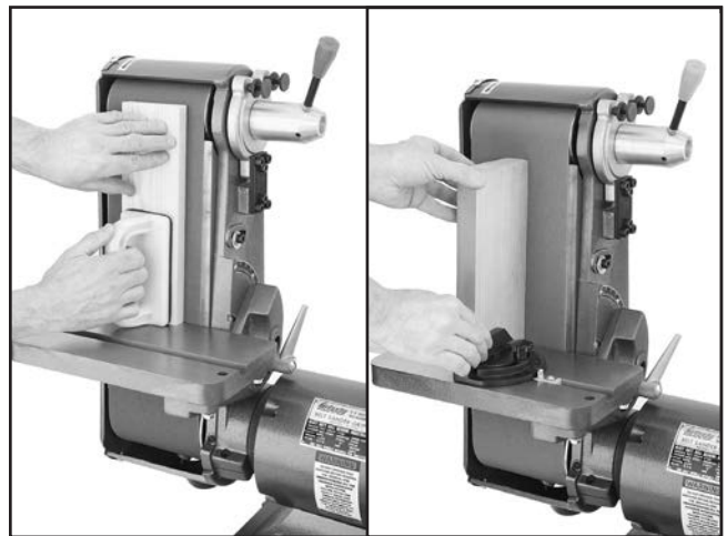
Figure 40. Examples of vertical face and edge sanding.
