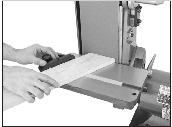
Figure 39. Example of vertical miter sanding.
