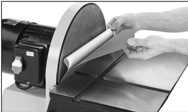
Figure 31. Example photo of installing the sandpaper disc.
