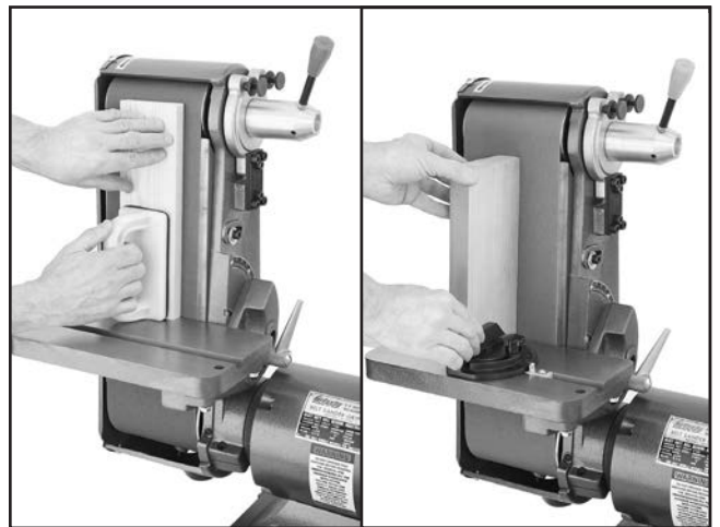
Figure 40. Examples of vertical face and edge sanding.
