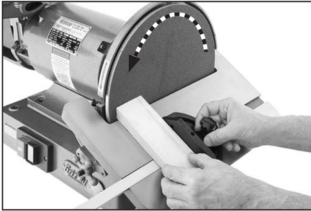
Figure 34. Example of compound angle sanding.
