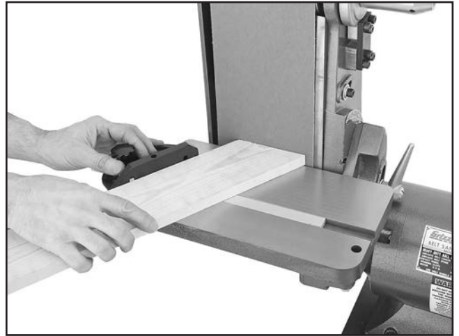
Figure 39. Example of vertical miter sanding.
