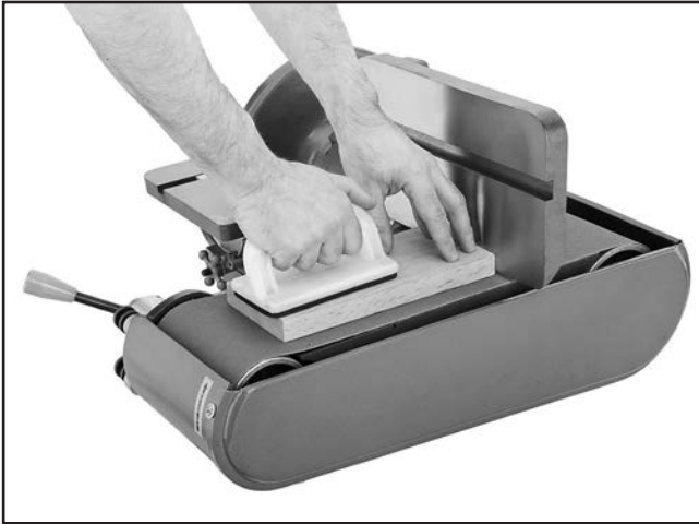
Figure 37. Sanding workpiece in horizontal position.
