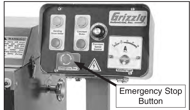
Figure 18. Location of Emergency Stop button.
