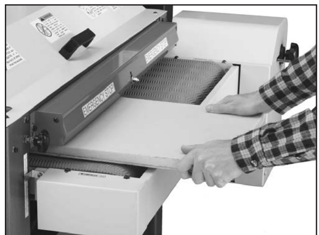
Figure 32. Example of using D3003 PRO-STIK® Cleaning Pad to clean sandpaper.
