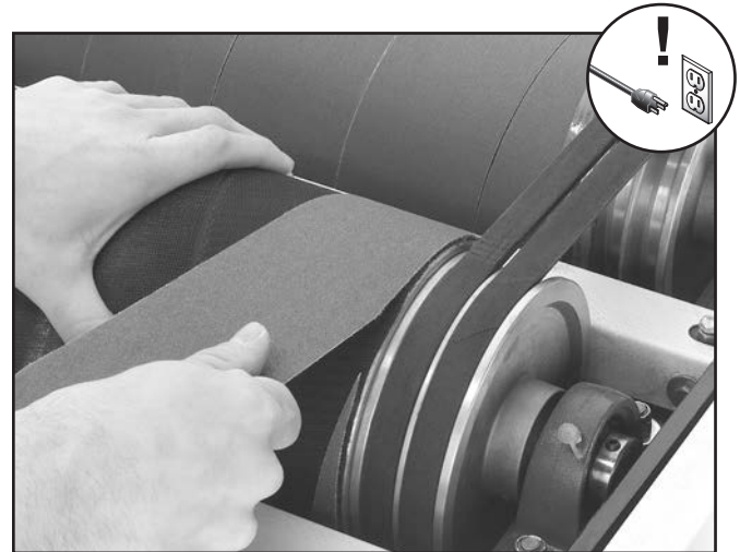
Figure 28. Example of wrapping sandpaper around drum.
