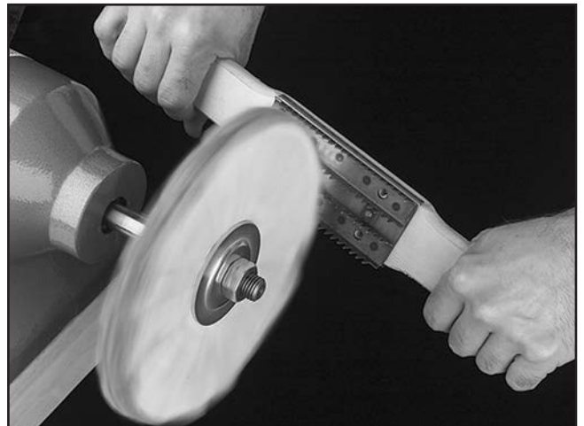
Figure 14. Removing compound from buffing wheel with buffing wheel rake.
