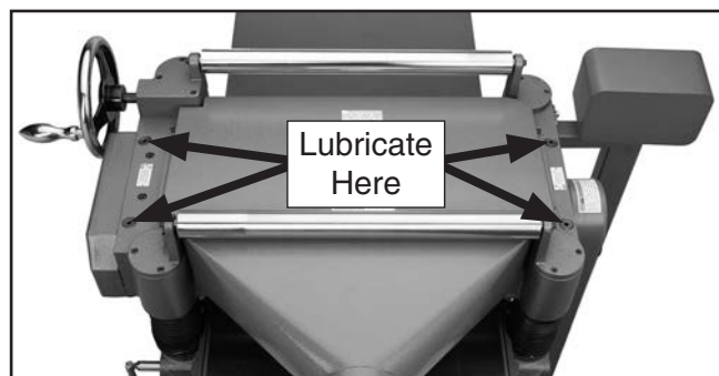
Figure 40. Lubrication locations for feed roller bushings.
