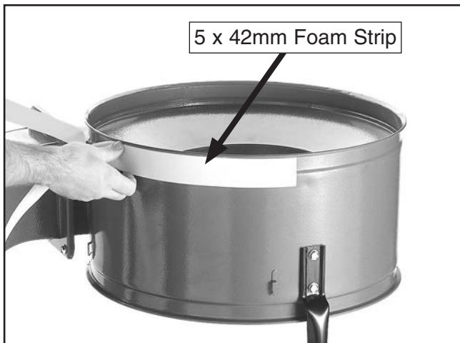
Figure 30. Example of applying the wide foam strip to the collector.
