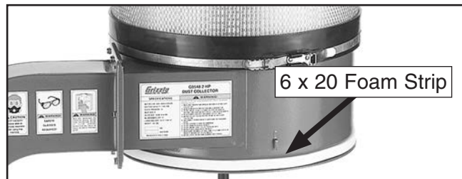
Figure 34. Example of 6 x 20 foam strip installed.
