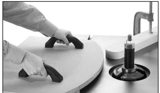
Figure 52. Use starting pin substitute when needed. (Guard removed for clarity.)
