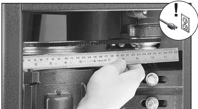
Figure 72. Checking pulley alignment.
