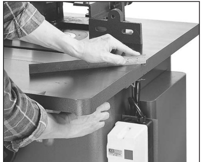
Figure 20. Adjusting to ensure flatness.
