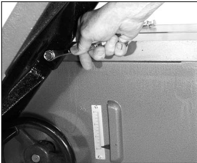
Figure 19. Installing extension wing.
