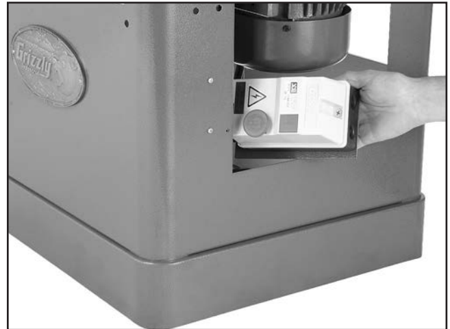
Figure 9. Removing magnetic switch from cabinet.
