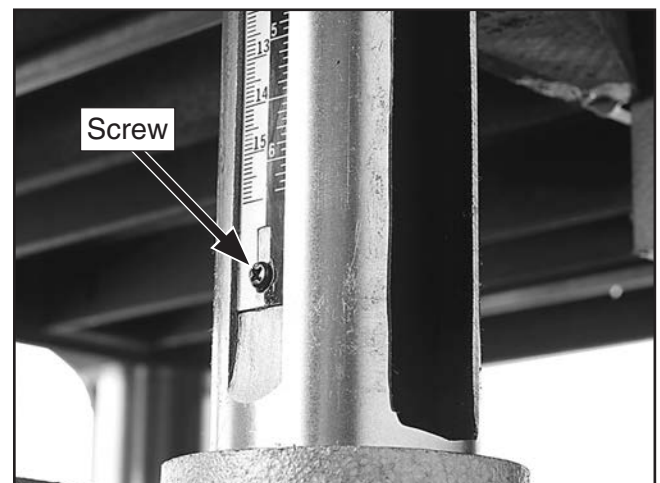
Figure 63. Location of adjustment screw for table elevation scale.
