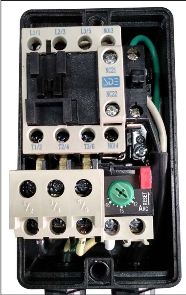
Figure 72. G1021Z magnetic switch with cover removed.
