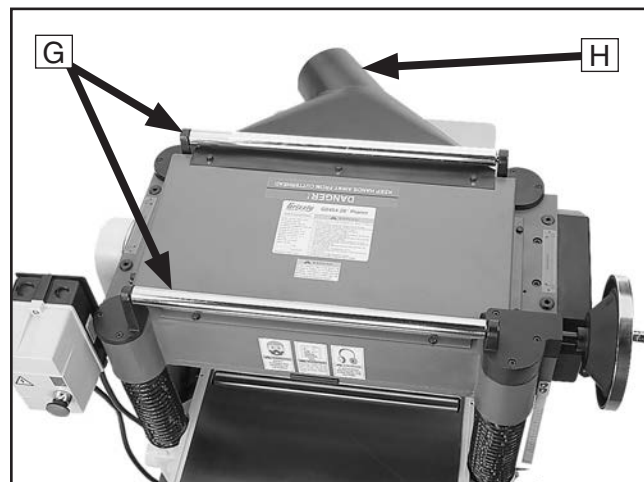
Figure 2. Example of return rollers and dust port.
