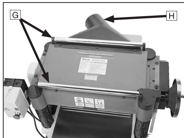
Figure 2. Example of return rollers and dust port.
