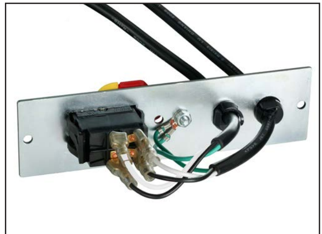
Figure 92. G1014Z switch wiring.
