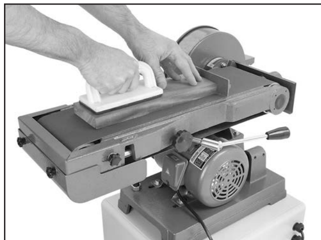
Figure 54. Sanding workpiece in horizontal position.
