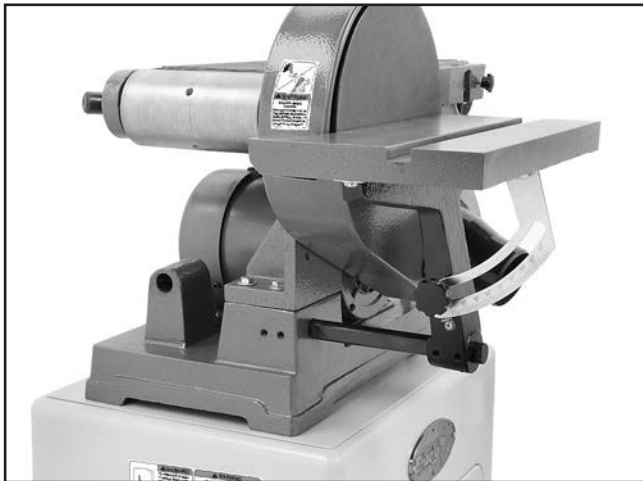
Figure 36. Installing work table onto table support rod.
