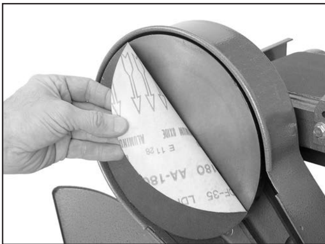
Figure 32. Installing sanding disc onto cast iron plate.
