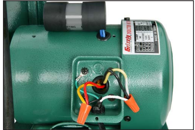
Figure 91. G1014Z 110V motor wiring.
