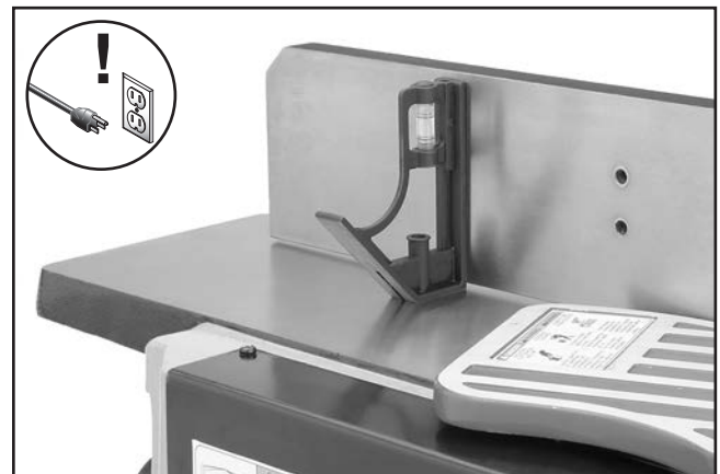
Figure 53. Example of checking 90° fence angle with square.
