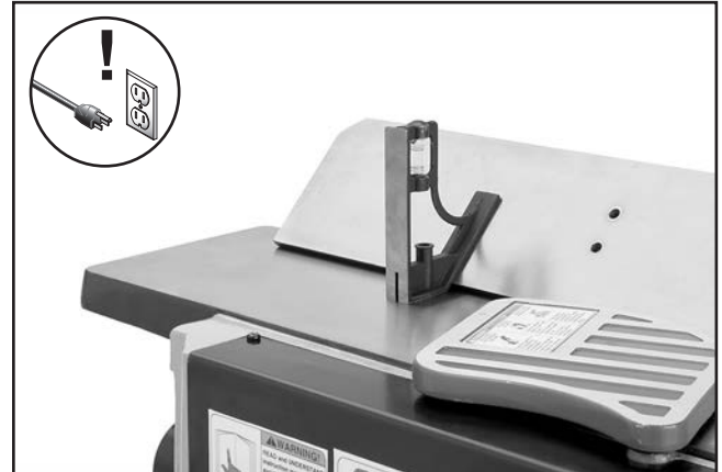
Figure 56. Example of checking 45° fence angle with square.
