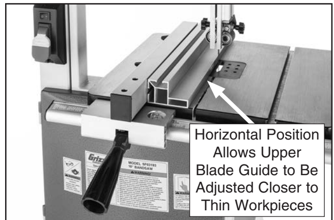
Figure 3. Fence mounted in horizontal position.
