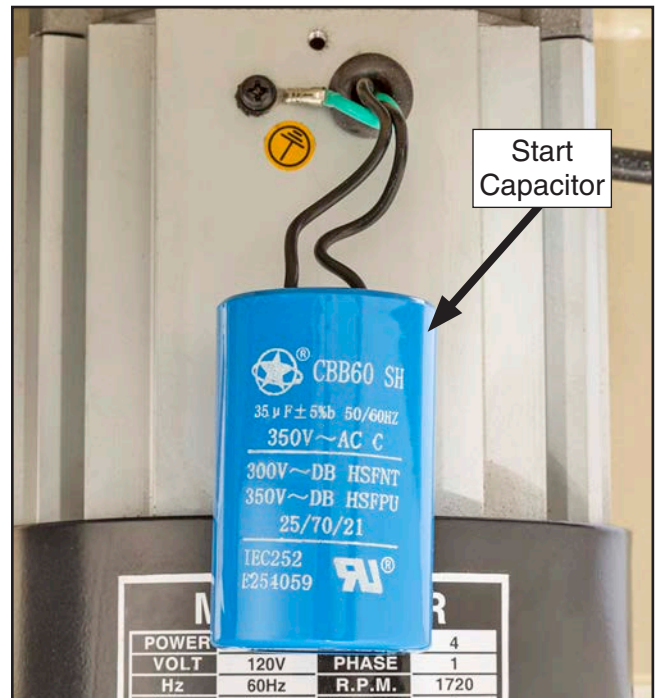
Figure 78. Start capacitor wiring.
