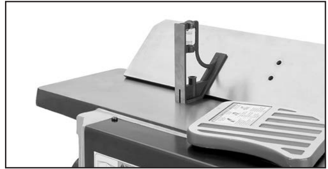
Figure 59. Example of checking 45° fence angle with combination square.
