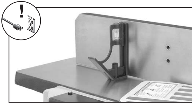
Figure 57. Example of checking 90° fence angle with combination square.
