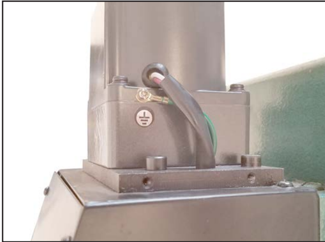
Figure 74. Z-axis motor wiring.
