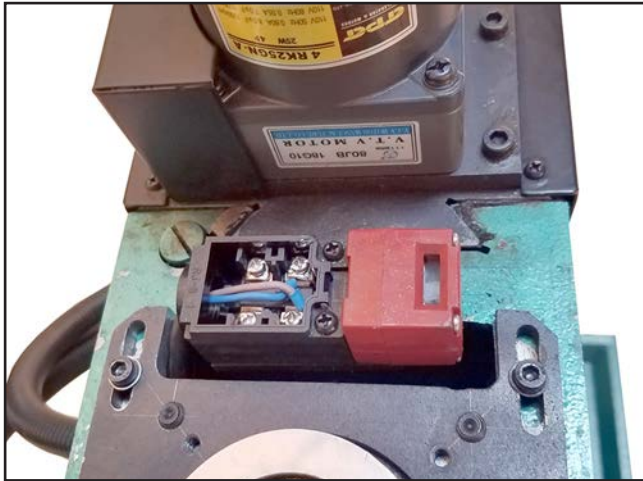
Figure 80. Headstock cover safety switch wiring.
