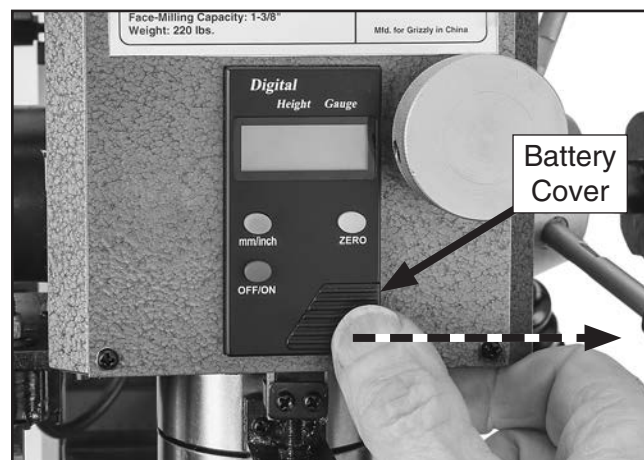
Figure 58. Battery cover for spindle depth DRO.
