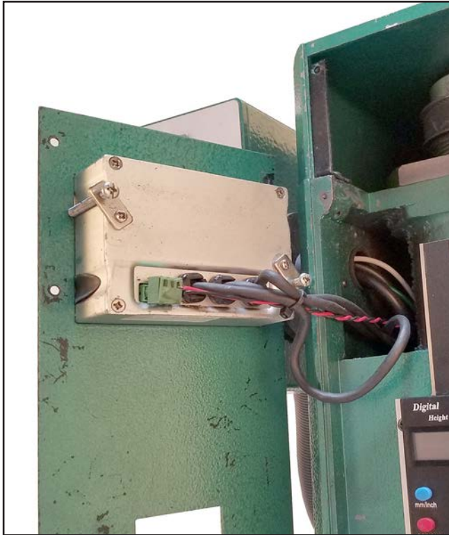
Figure 77. 3-axis DRO and spindle depth DRO wiring.
