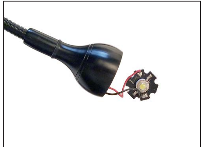
Figure 81. LED worklight wiring.
