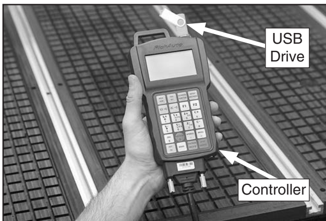
Figure 62. USB drive connected to controller to upload G-code to controller.
