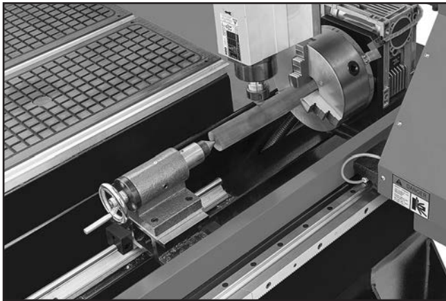
Figure 60. Spindle \frac{1}{8} " above workpiece toolpath origin.
