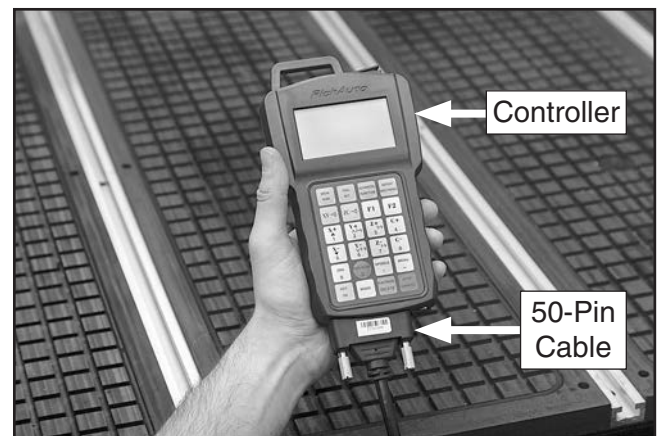
Figure 25. Controller connected to cable.
