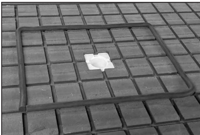
Figure 50. Example of gasket tube cut to size to seal workpiece to vacuum zone.
