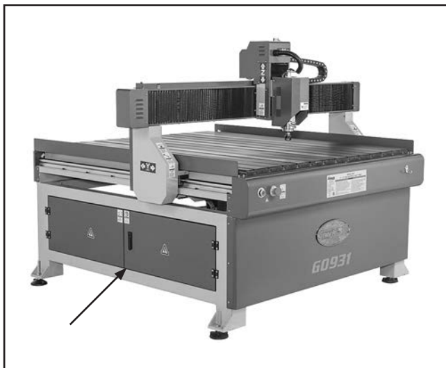
Figure 13. Electrical cabinet location.
