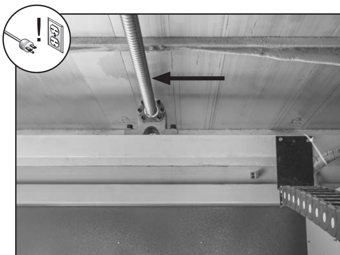
Figure 38. Y-axis ball screw lubrication area.
