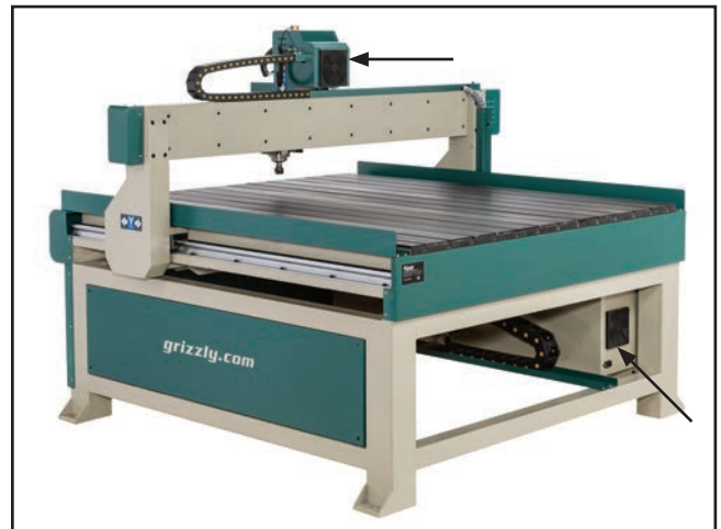
Figure 53. Electrical cooling fan locations.
