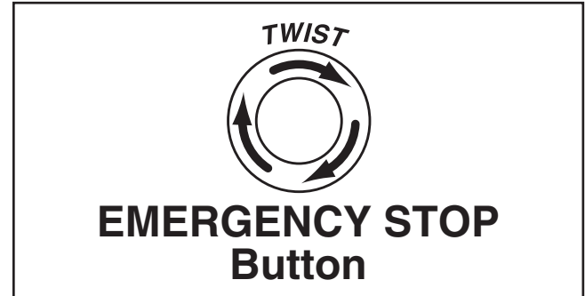
Figure 18. Resetting EMERGENCY STOP button.
