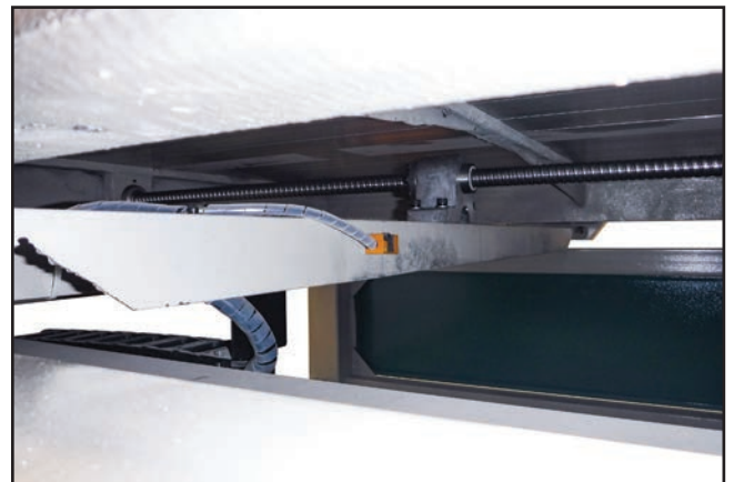
Figure 60. Y-axis limit switch.
