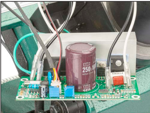
Figure 62. Circuit board wiring.
