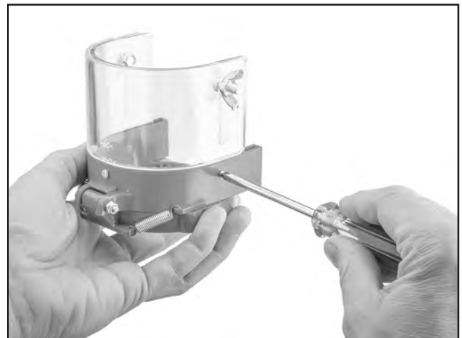
Figure 4. Attaching chuck guard to chuck guard seat.
