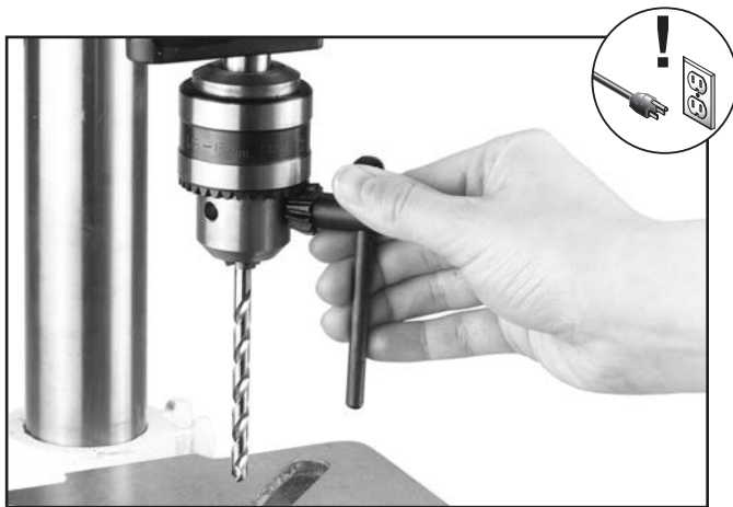
Figure 21. Example of tightening chuck with chuck key.
