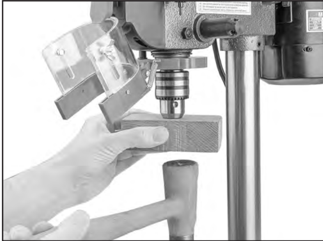
Figure 9. Using block of wood and hammer to tap chuck onto spindle taper.
