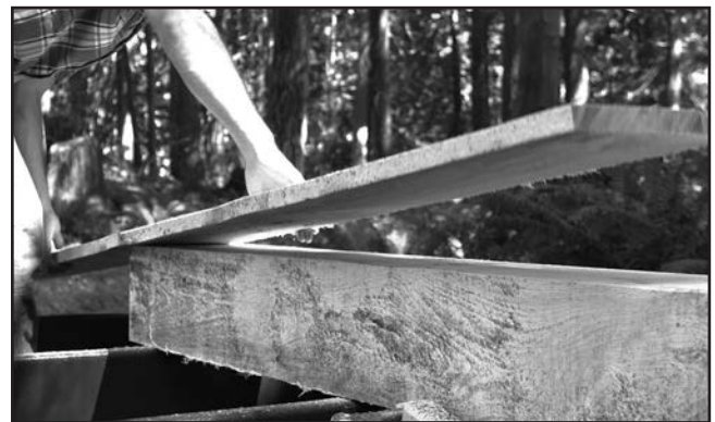
Figure 40. Example of live sawing a cant into dimensional lumber.
