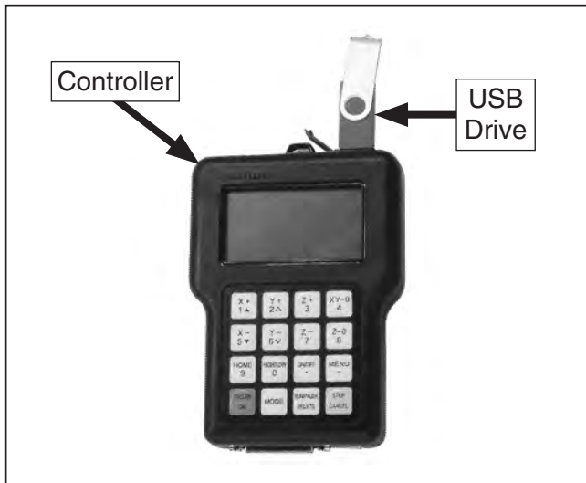
Figure 45. USB drive connected to controller.
