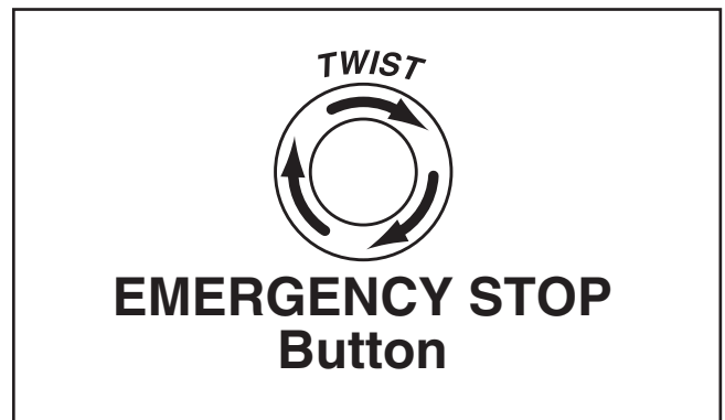
Figure 35. Resetting the EMERGENCY STOP button.
