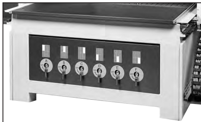
Figure 42. Vacuum zone control valves.
