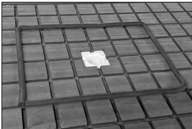
Figure 41. Gasket tube cut to size to seal workpiece to vacuum zone.
