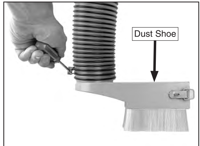
Figure 26. Tightening dust hose clamp.
