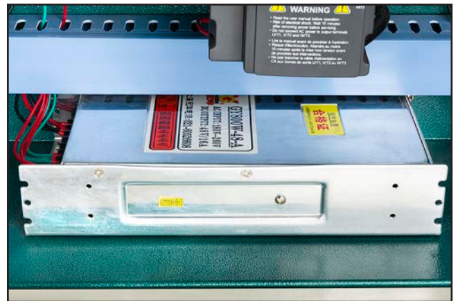
Figure 34. 48-Volt power supply.
