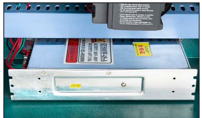
Figure 34. 48-Volt power supply.
